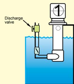
Solution level above impeller. Suction head available
